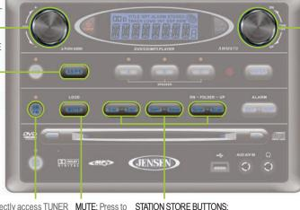
TUNE/TRACK: Rotate COUNTER CLOCKWISE to TUNE DOWN in frequency. Rotate CLOCKWISE to TUNE UP in frequency. Rotate and hold to scan to next strongest station.
